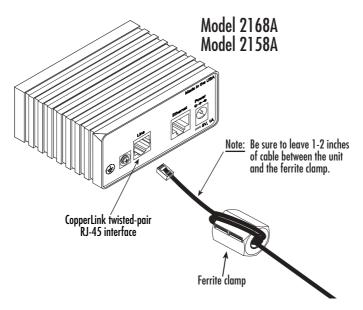
Figure 5. Connecting the ferrite clamp for 2168A/2158A models
